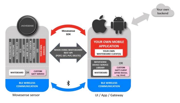
Figure 6 Movesense Architecture. Source (Movesense, 2021)
