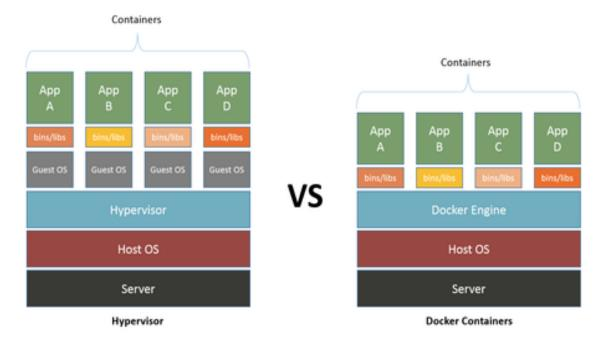
Figure 8 Hypervisor vs Docker container (Source: Network Computing, 2021)
