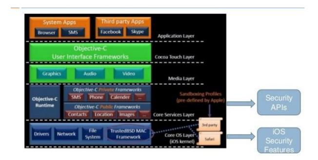
Figure 21 iOS Software Stack (Source: Ahmed-Reza Sadeghi et al)
