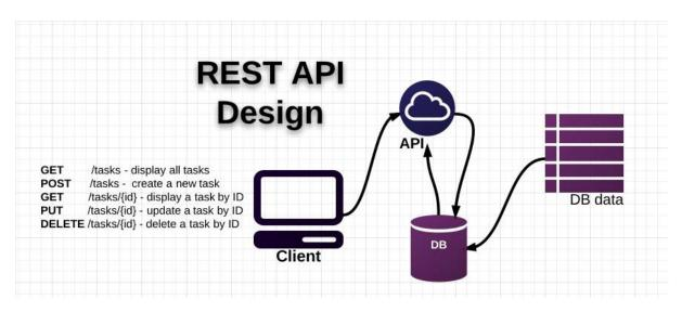
Figure 12 REST Architecture (Source: maxoffsky.com)
