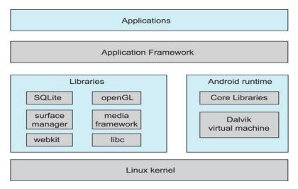
Figure 20 Android OS Software Stack (Source: Operating System Concepts)
