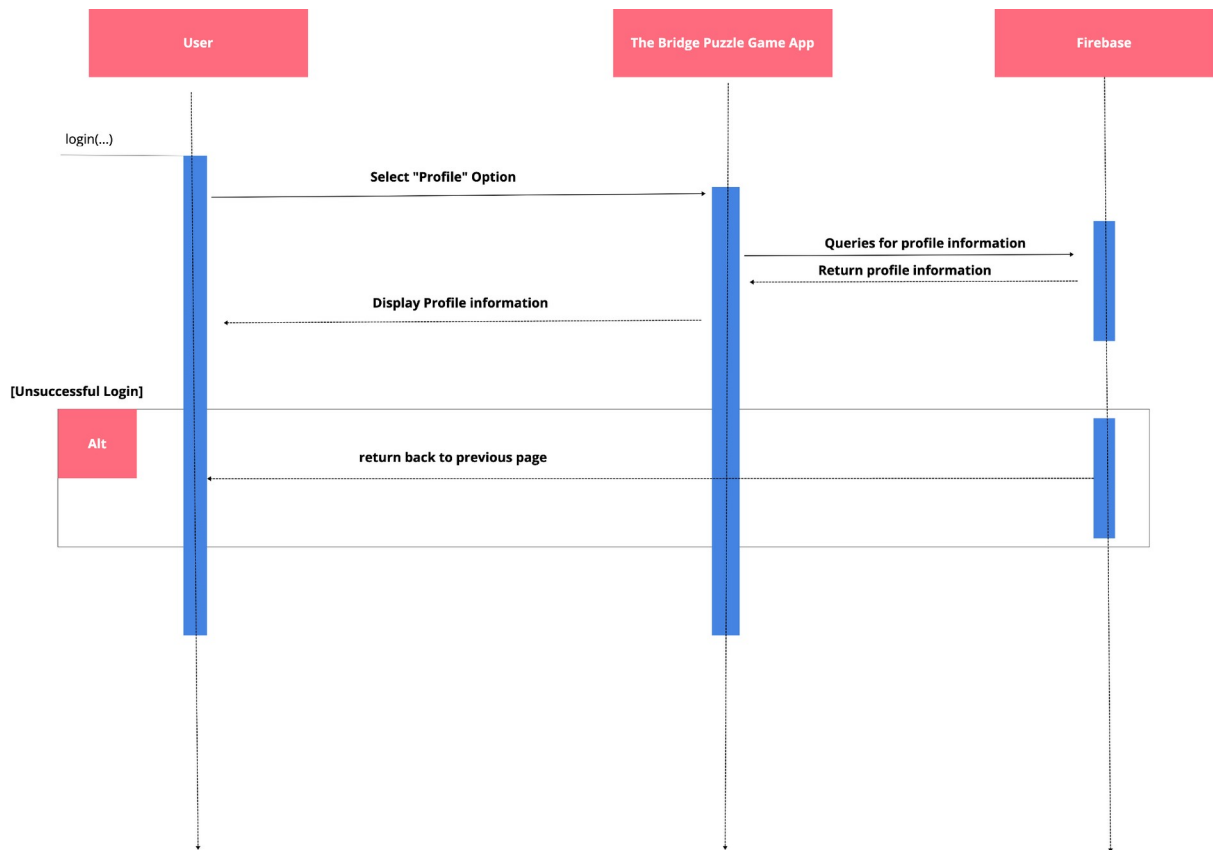
Figure 7 Sequence Diagram - View Profile
