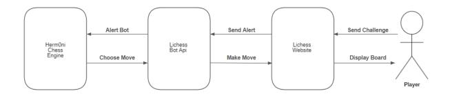
This context diagram shows the communication flow from the user to the engine through the lichess.org website and the lichess bot API.
